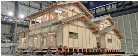
Full-scale earthquake testbed of a traditional wooden house of two stories with an attached upper unit (2012, E-defence)
